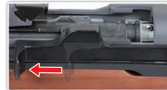
Pulling the bolt handle backward to reveal the hop-up unit.
